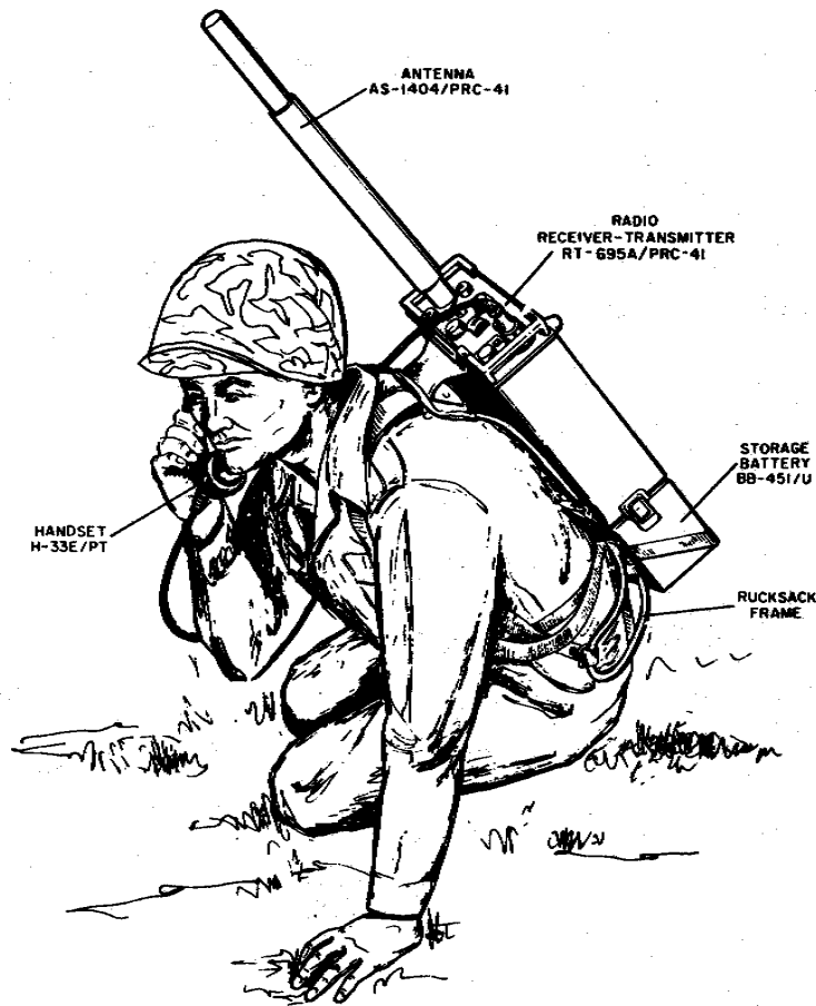
Figure 2-4. Radio Set AN/PRC-41A, Man-Pack Installation
